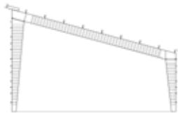
**VILNIUS** A framework for buildings with mono-pitched roof such as wood stores, garages or simpler machine halls. The frame is also suitable when the slope of the roof is required in a certain orientation.
